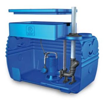
Prefabricated **lifting stations** are an effective, economical solution for collecting domestic wastewater and transferring it to a sewer at a higher level or where there are barriers to gravity run-off, or where the wastewater requires grinding.
