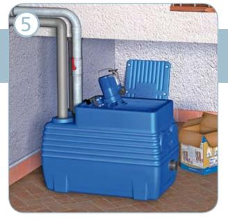
The next step is to install the pump, which will certainly be easier if a BlueBOX with DAC was chosen. In this case, the flange provided has only to be slid along the guide tubes to achieve perfect coupling to the body of the DAC.
