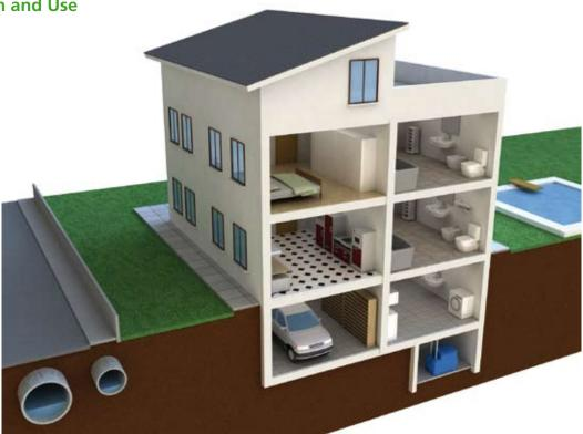
The collection tank receives household wastewater from drains of any kind, and any rainwater or seepage drains. The pump installed inside the tank refluxes the wastewater into the sewer.
