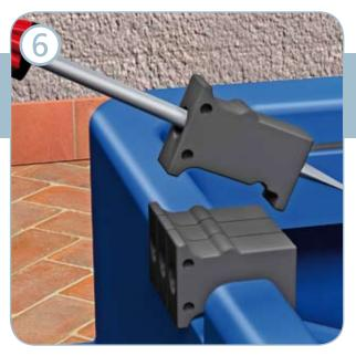
The electrical cables are passed through special patented rubber cable glands that ensure a perfectly airtight seal. Before fitting the cable, perforate the chosen cable glands with a sharp tool, but leave the others intact to keep liquids or smells inside the unit.
