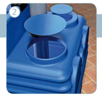
Before the unit is actually placed in position, holes are drilled in the sides using a flared grinding tool to take the seals and then the pipes in the chosen positions.
